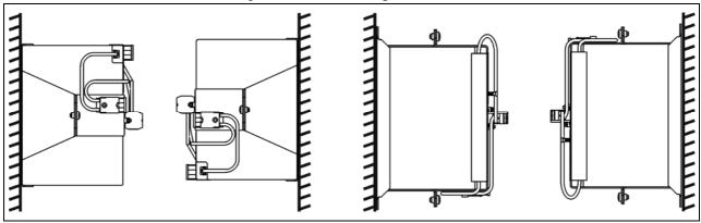
Do not use the battery module in an upside down position:
